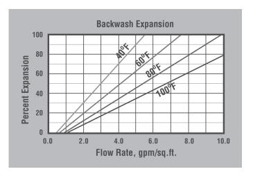
**BACKWASH** — After each cycle the resin bed should be backwashed at a rate that expands the bed 50 to 75 percent. This will remove any foreign matter and reclassify the bed.
