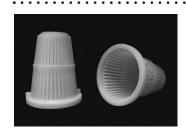
**SWT's Upper Screen/Diffusers** can be cemented to a valve or tank head, or fixtured with two 3/32 inch self-tapping screws. *Total open area of slots: 1.070 sq.in.*
