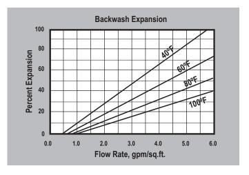
**BACKWASH** — After each cycle the resin bed should be backwashed at a rate that expands the bed 50 to 75 percent. This will remove any foreign matter and reclassify the bed. The graph above shows the expansion characteristics of ProSoft ER10011-NA in the hydrogen form.
