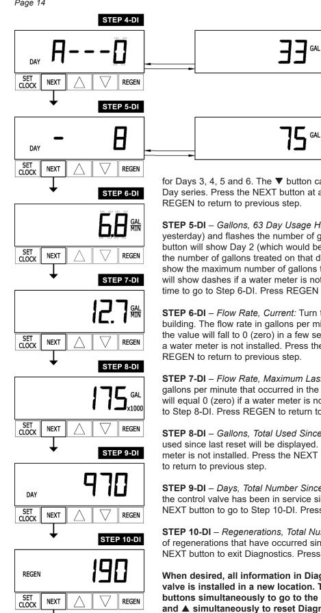
STEP 4-DI – Gallons, Reserve Capacity Used for Last 7 Days: If the valve is set up as a softener, a meter is installed and Gallons Capacity (Step 7-SS, Page 9) is set to "Auto", this display shows Day 0 (for today) and flashes the Reserve Capacity. Pressing the button will show Day 1 (which would be yesterday) and flashes the Reserve Capacity used. Pressing the ▲ button again will show Day 2 (the day before yesterday) and the Reserve Capacity. Keep pressing the **▲** button to show the gallons
