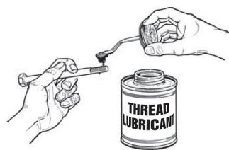
**STEP 1** Use of well lubricated bolts & flat washers are required. Use an anti-seize lubricant such as IMS Copper Flake.
