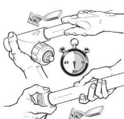
Allow joint to cure according to solvent cement manufacturer's instructions.
