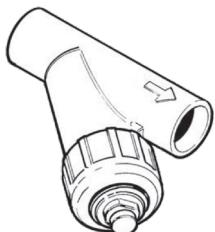
Resin traps may be mounted in either horizontal or vertical positions. However, attention should be paid to flow direction as indicated on the strainer body. The strainer basket should be pointed downward to properly collect sediment and facilitate flushing.
