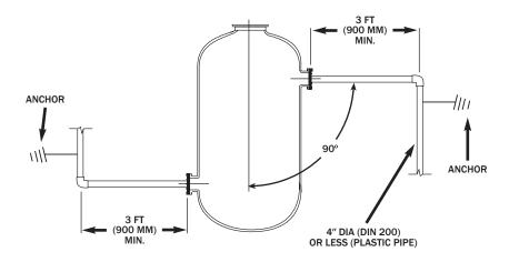
The figures shown here are the acceptable minimum for the pressure vessel at its rated pressure of 150 psig. When using the pressure vessel at a lower pressure, the minimum pipe run length can be reduced, using this formula:
