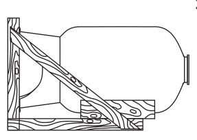
1. When delivered, the pressure vessel and skid may be in a horizontal position. The first step is to stand the whole assembly upright. All precautions described earlier should be observed to protect the pressure vessel from damage.
