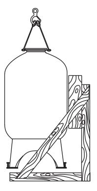
**4.** Lower the pressure vessel to the floor, level the pressure vessel, and anchor it with 3/8 inch lag bolts to the floor.
