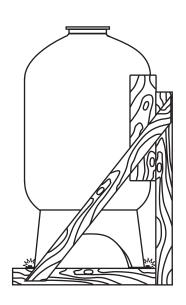
2. When the pressure vessel and skid are upright, **remove the lag bolts** which are holding the skid to the base of the pressure vessel.
