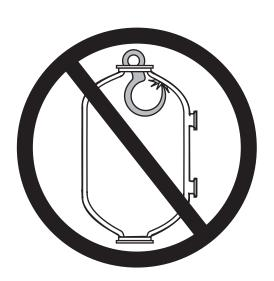
**6.** Avoid use of hooks or equipment on the **inside** of the pressure vessel.
