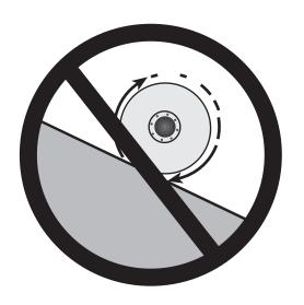
**2.** Never roll or slide a pressure vessel on its side.
