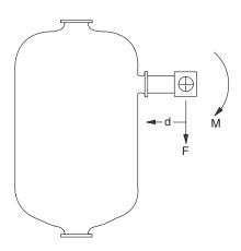
Valves, piping, and hardware all contribute to the weight loads put on side flanges. Side flanges are rated for a maximum bending torque (M) of 50 ft-lb. This means that:
