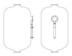
To support greater loads, a support kit is available for upper side flanges only. With the support kit, the side flange is rated for a bending torque (M) of 300 ft-lb.
