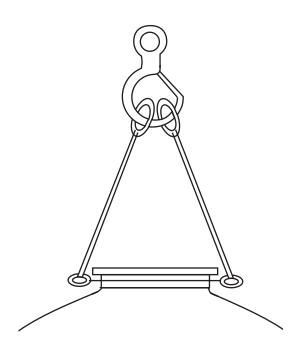
8. Never fasten cables or chains around pressure vessel.
