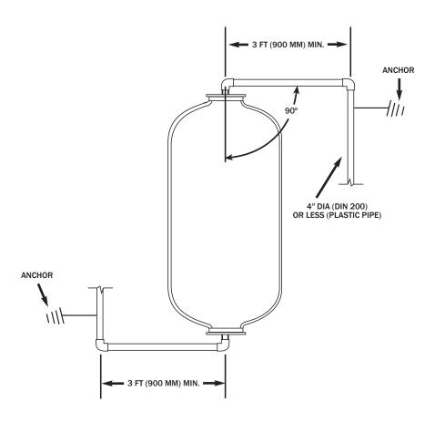
An effective alternative to flex connectors uses the inherent flexibility of right angle system design. By calculating the amount of cantilever overhang needed to absorb the torsional effect created by the pressure vessel's vertical movement, it is possible to build the needed flexibility right into the piping system. This can be done with both top/bottom and side flow piping setups.
